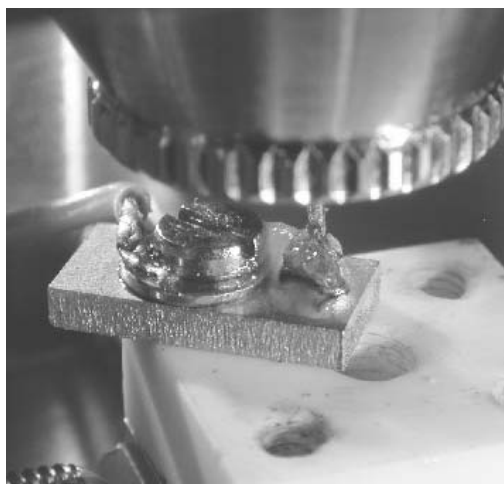
FIGURE 2. The tip and sample of our home-built STM immersed in a gel which allows scanning for several days at the gel-HOPG interface. In the center of the image we see the tip and the gel-covered HOPG.
