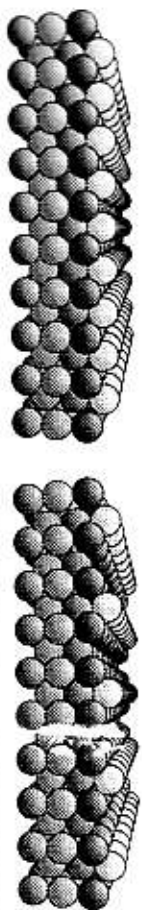
FIGURE 1: Model (perspective view) of a regular fcc (110) surface and of (1x2) reconstructed surface. The reconstructed phase has been named "missing row" structure.
