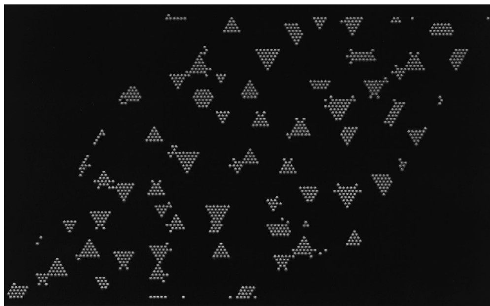
Fig. 8. ‘Snapshot’ from the simulation ( 200 \text{ \AA} \times 200 \text{ \AA} ) of the 2D triangular S islands produced by segregation.
