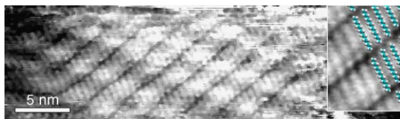
Fig. 1. Constant current image ( I = 10 pA, V = 300 mV) of Au(111) with a self-assembled monolayer of n -tetradecane. Both the reconstruction of the gold and the individual C_{14}H_{30} molecules are discernible. The inset shows a correlation averaged zoom-in, with some molecules drawn in to indicate the structure of the monolayer.
